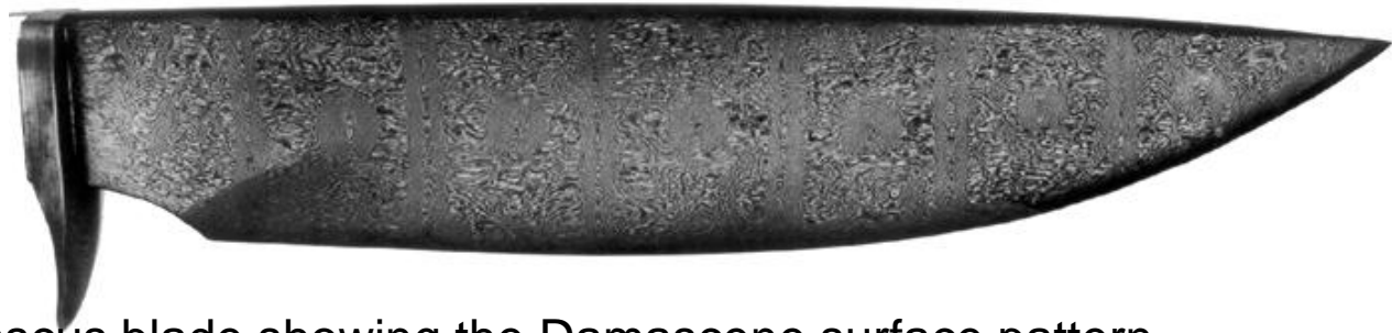
Damascus blade showing the Damascene surface pattern containing a combined Mohammed ladder and rose pattern
